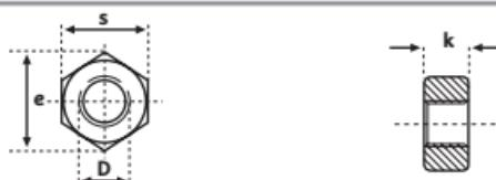
Metric threads, dimensions [mm] [DIN934]
